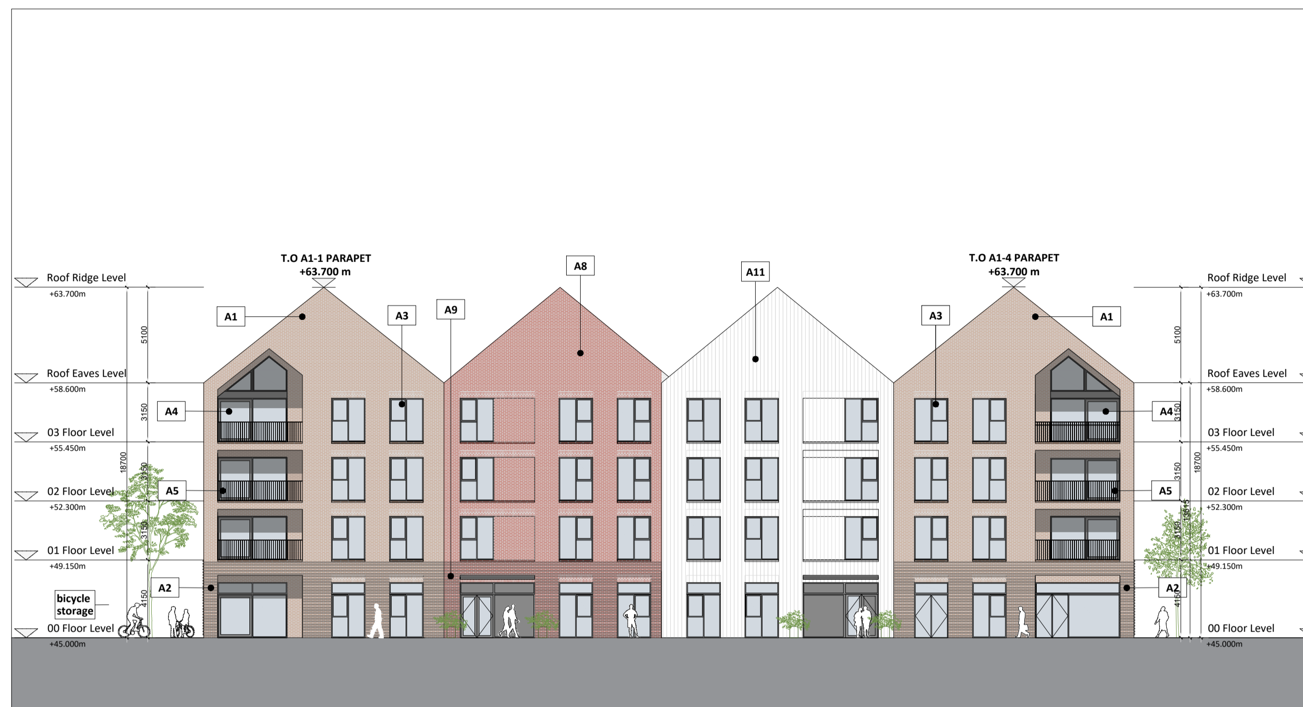
BLOCK 1 NORTH ELEVATION
